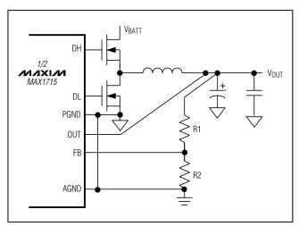
Figure 8. Setting V<sub>OUT</sub> with a Resistor-Divider
