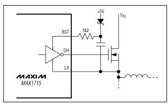
Figure 6. Reducing the Switching-Node Rise Time
