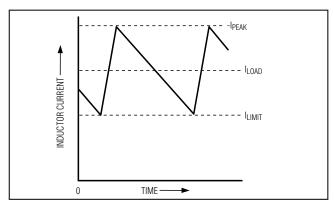
Figure 5. "Valley" Current-Limit Threshold Point
