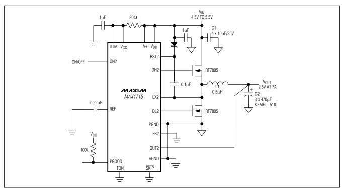
Figure 10. 5V-Powered, 8A CPU Buck Regulator
