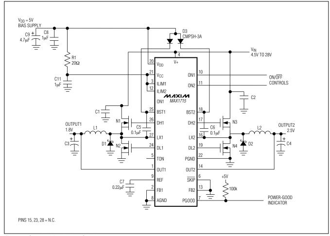
Figure 1. Standard Application Circuit
