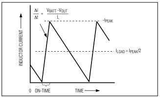
Figure 4. Pulse-Skipping/Discontinuous Crossover Point
