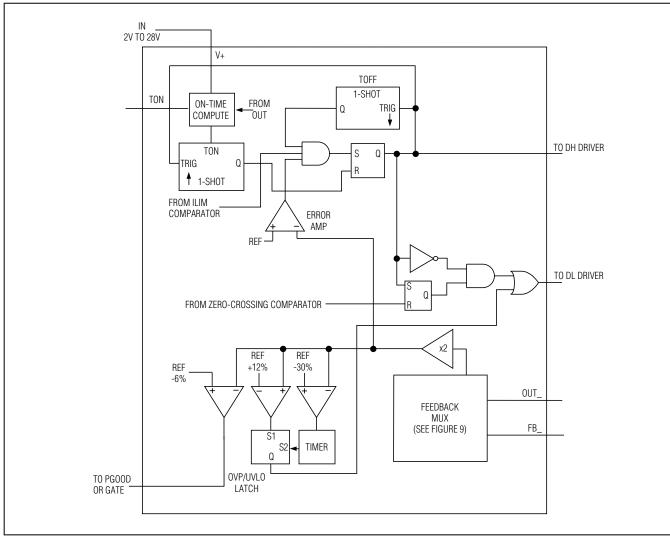
Figure 3. PWM Controller (one side only)
