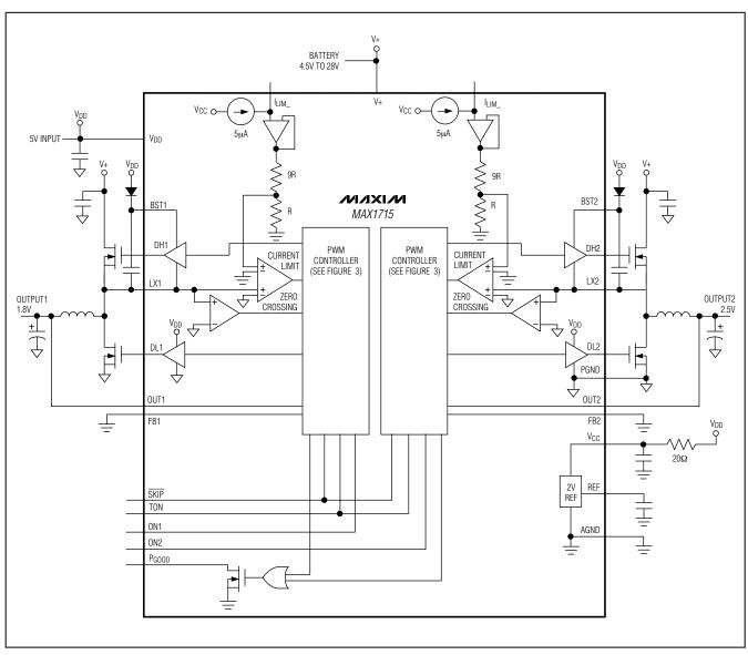
Figure 2. Functional Diagram
