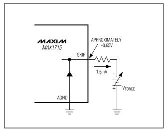
Figure 7. Disabling Over/Undervoltage Protection (Test Mode)
